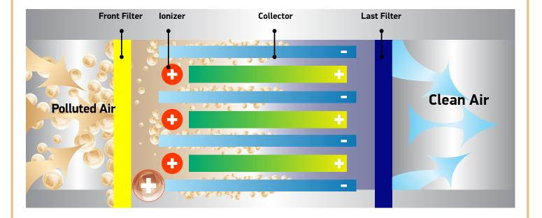
High voltage units that are used in our air cleaning plants are designed specially. These units work with 220 volts. They produce 20.000 – 100.000 high voltage with 100 watts and more energy. Thanks to their specially designed high voltage units, electrostatic filters makes high filtration.
